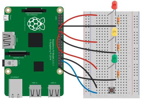
Next, set up the following trivial script in Scratch and run it. This will configure GPIO 16 as an input. We need to do this prior to using "sensing" blocks with the button:
